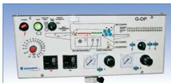
A line of fusing presses suitable for middle and big size companies, who are looking for perfect quality fusing and max productivity. Available in 5 widths (75, 100, 112, 140 and 160 cms). Uniformity of heating is obtained by the instantaneous heating system of 4 upper elements and 5 lower elements. Complete of electronic control panel for displaying ; fusing temperature (upper and lower), speed in m/min or sec, rollers pressure, ZERO pressure device, faults prevention.
