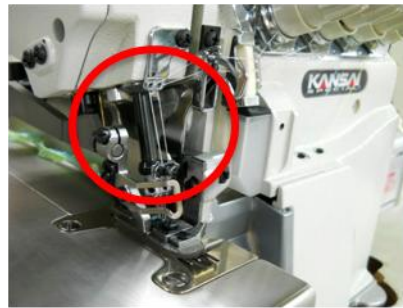
■ Diamond Like Carbon(DLC) coated needle bar and upper looper holder Ensure durability and reliability.
