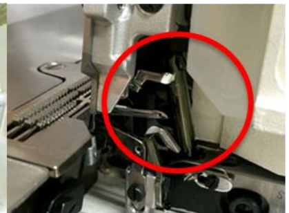
■ Diamond Like Carbon(DLC) coated needle bar and upper looper holder Ensure durability and reliability.
