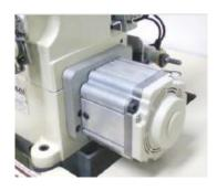
Option: direct drive servo motor increases productivity and saves electricity cost
