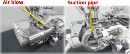
Air blower to folding area avoids fabric from curling as well as to help send excess fabric to suction pipe.
