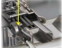
Carbide knife ensures clean cut and durability.
