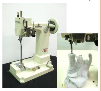
Original Kansai looper that provides a consistent stitch, with one screw maintenance and no adjustment.
